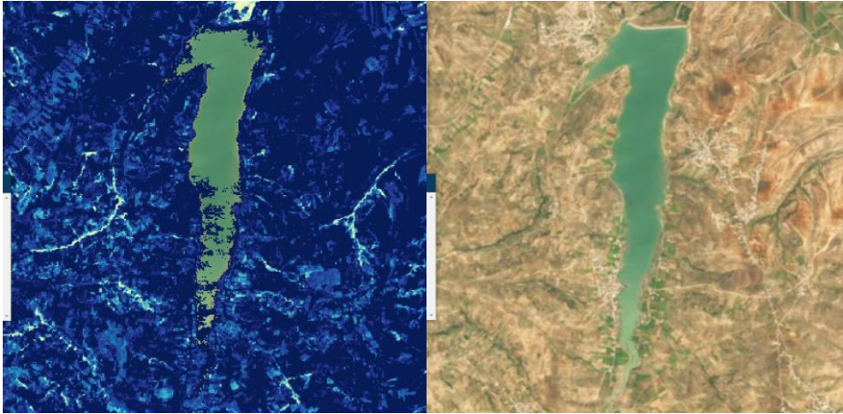
Figure 12: Water mask in Syria data cube, AOI Yarseli Bajaji.
